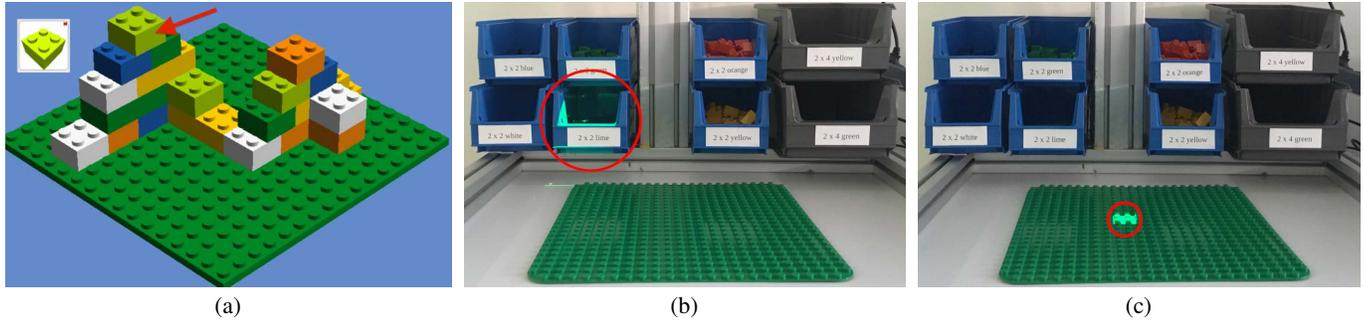
Figure 2. Used assembly instruction systems. (a): Printed *paper instruction*. (b): *In-situ projection* highlighting an item bin. (c): *In-situ projection* indicating where to put the Lego Duplo brick.
